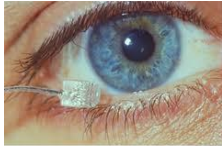
The artificial retina consists of an electrode-studded silicon chip (shown) that is tacked to the retina inside the eye.
